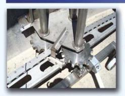
The patented traction system of the BTEC models guarantees total stability in the rotation of the bearing ring thanks to the 3 driving gears.
