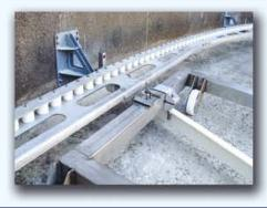
The bearing sing slides along self-adjustable support guides.
